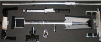
These kits contains all the torque wrenches and associated support equipment for securing the Universal Joint bolts and fixings to the correct torque. These kits are for both KIT09001 and KIT09002 technology.
