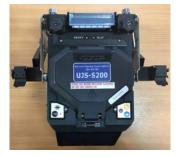
of the many fibre types. The kit also contains the cleaver which cleaves the fibre end to a high degree of precision and the printer, which provides a written record of the splice data. The splicer contains a built-in oven for shrinking the heat-shrink fibre splices once completed.
