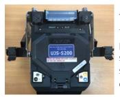
The kit also contains the cleaver which cleaves the fibre end to a high degree of precision and the printer, which provides a written record of the splice data. The splicer contains a built-in oven for shrinking the heat-shrink fibre splices once completed.
